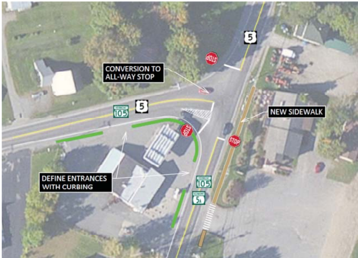
Figure 53: US 5/VT 105 Intersection All Way Stop Design Plan
