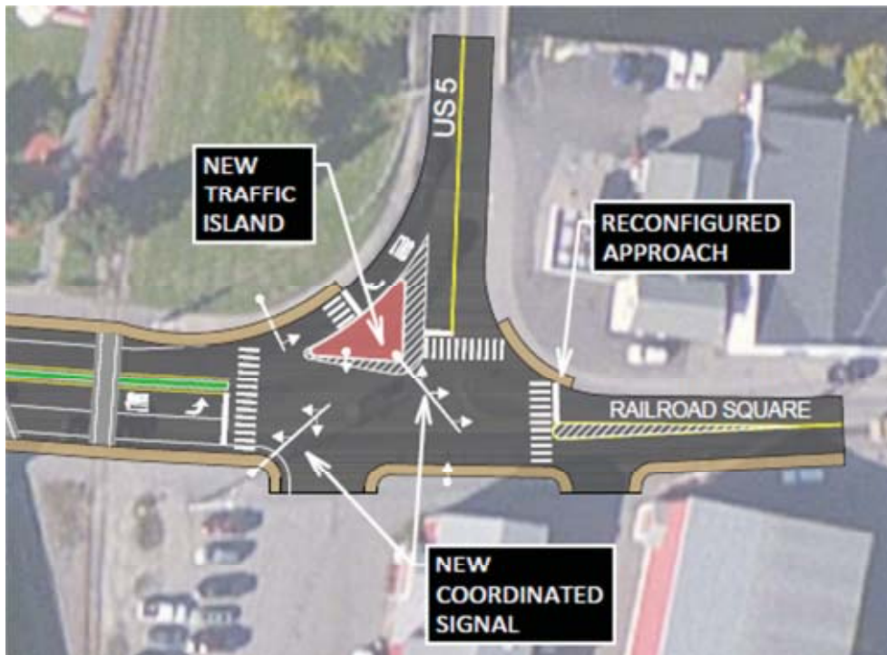
Figure 49: Railroad Square Intersection Signalization Design Plan
