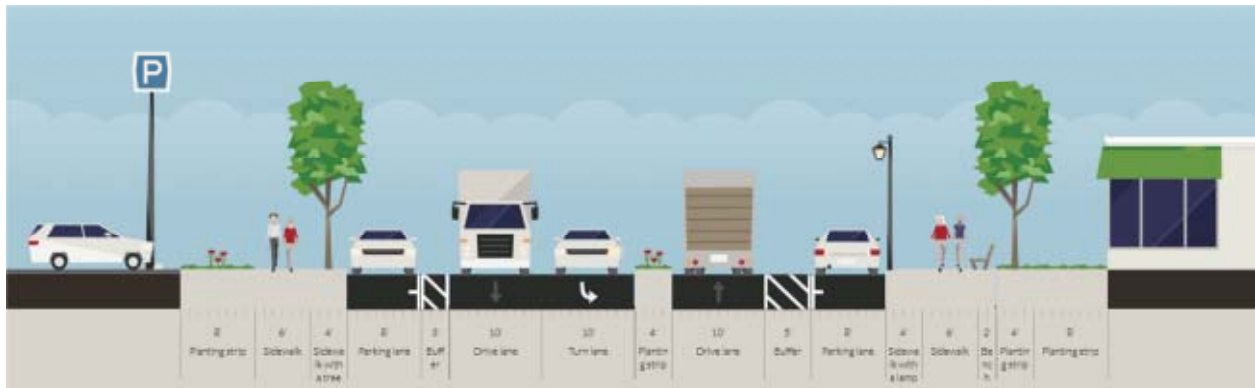
Figure 47: Proposed US 5 Cross-Section between Coventry Street and Railroad Square
