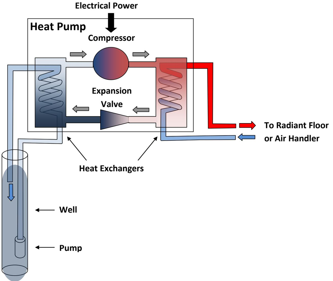
Here, well water is pumped through a heat exchanger, where heat flows from the well water into the cold refrigerant. The refrigerant is then compressed, which greatly raises its temperature. The refrigerant, which is now hot and vaporized, then loses its heat in the second heat exchanger to water which is then circulated either under a radiant floor or into an air handler.
