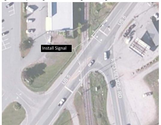
Figure 62: US 5/Red Village Road Intersection Signalization Diagram
